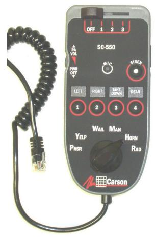
The SC-550-10CH Hand Control has the same modular plug that is used on the re-designed Hand Control for the SC-550-83 Model. The earlier SC-550-83 Models have a circular DIN connector for the hand control. The earlier SC-550 Model will need to be upgraded with the rectangular modular connector to use SC-550-10CH Hand Control.
